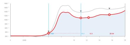
The RULERTM View generates a voltammogram, identifying the type and quantity of healthy antioxidants in the lubricating oil or grease. This information provides a window into the Remaining Useful Life of your lubricant.
